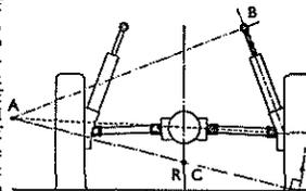
The geometrical construction for determining the position of the roll centre of the rear suspension.
